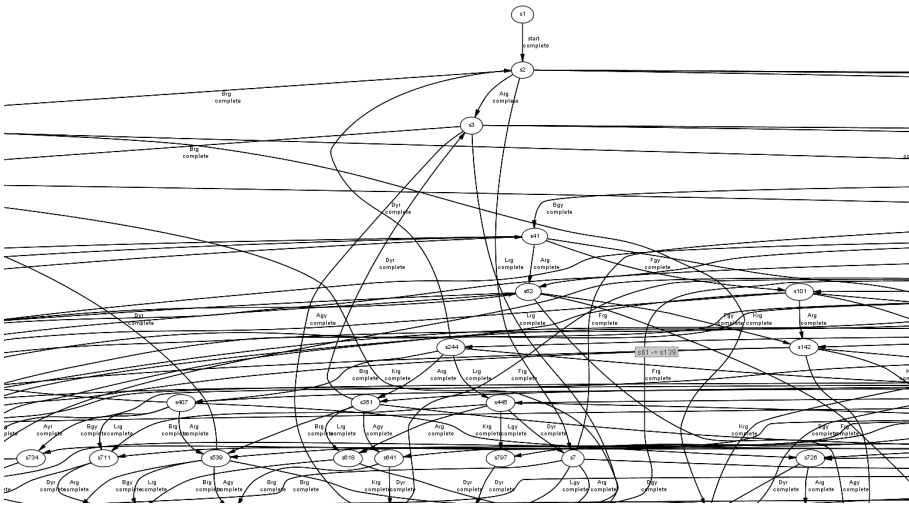
Fig. 9. A visualization of a fragment of the entire state space for the traffic light controller
